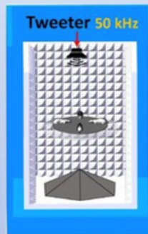
60 dB Sound-isolation Chamber
